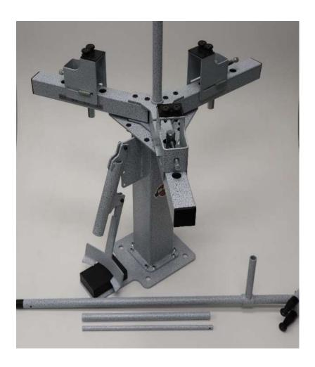
Note regarding Center Post Selection: The three (3) included center posts are approximately 1/2" (13mm), 3/4" (20 mm), and 1" (26mm) wide. Use the largest center post you can fit through the bearing or opening in your wheel for maximum leverage when mounting and demounting tires.
