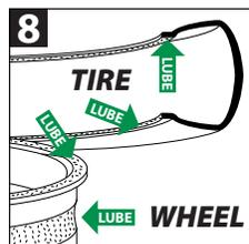
8 Wipe all spray lube from wheel and clean bead sealing surfaces thoroughly. Verify that wheel is still properly clamped in machine.
